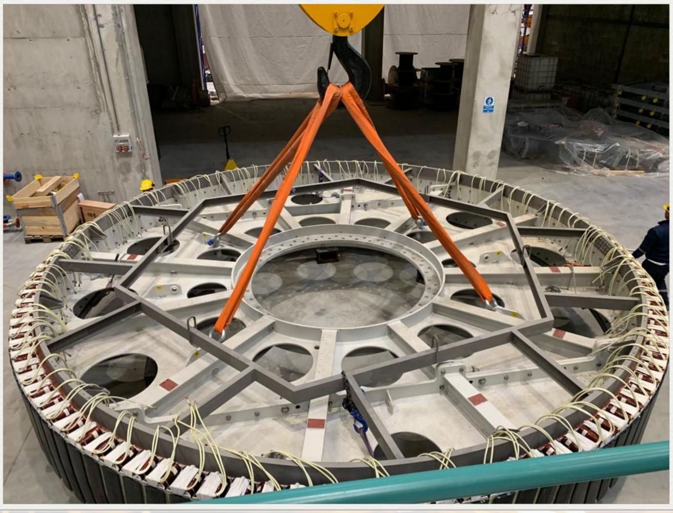
Mounting Parts of Wind Turbine Generator Manufacturing
